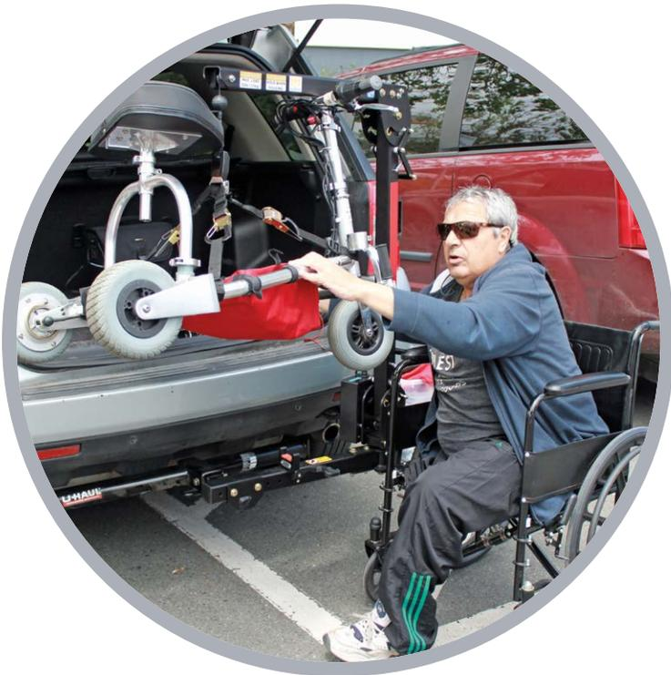
Dick was unable to go out in the community without a family member or friend to help him get his scooter in and out of his vehicle. So CanAssist provided him with the Hitch Lift, a battery-operated device that enables individuals to independently load a manual wheelchair, lightweight scooter or other mobility aid into a vehicle with very little physical effort or bending. Now, Dick is out on his own every day.
